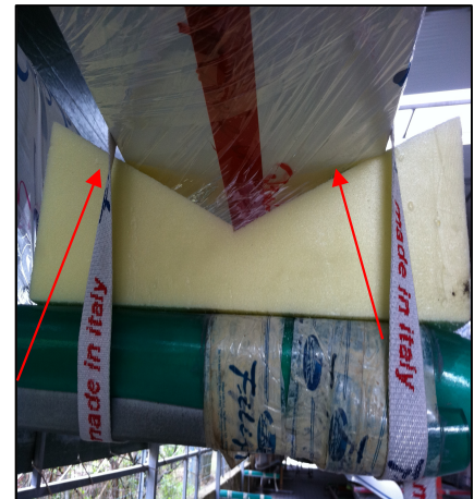
Correct shape of the foam supports: note the very limited areas of contact
